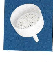
**BUCHNER FUNNEL Buchner with Stem,** fixed perforated plate, glazed inside and out except for rim
