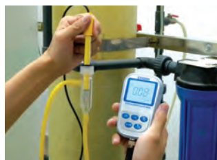
Conductivity/Resistivity Measurement of High Purity Water
